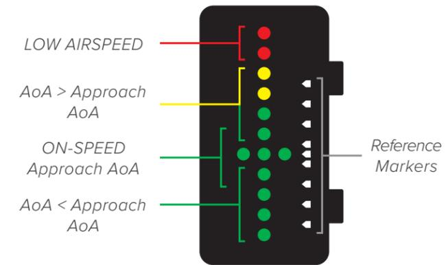
An Angle of Attack System is standard on all Skyhawks, delivering precise information for increased stall awareness, low-speed maneuvering capability and consistent maneuvers during takeoff, climb, cruise, approach and landing.
