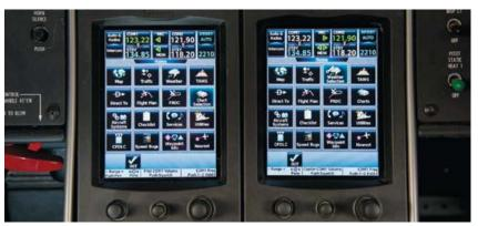
The GTC 570, an all-new glass touch-screen controller, is the primary connection for the Garmin G3000 system. This icon-driven interface enables you to access more systems and sensors than ever before. Functions are easy to locate with fewer touch points, allowing you more time heads up, looking forward.
